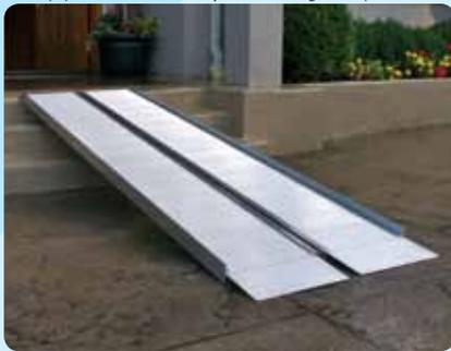
Features an extruded non-skid tread for superior traction, and a self-adjusting bottom transition plate for easy conversion from ramp to ground. Welded construction provides long-term durability and safety. Unfolds to a 30" wide platform. Top Lip Extension (TLE) compatible. 800 pound *bariatric* weight capacity.
