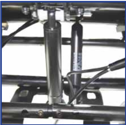
Dual cross gas cylinders to recline wheelchair with ease
