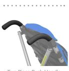
Two Piece Push Handle (Option) or Angle Adjustable One-Piece Push Handle (Standard)
